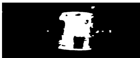
Fig. 13. Dilation and the erosion of the binary thresholding image.
